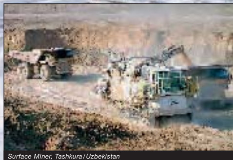
Surface Miner, Tashkura / Uzbekistan
